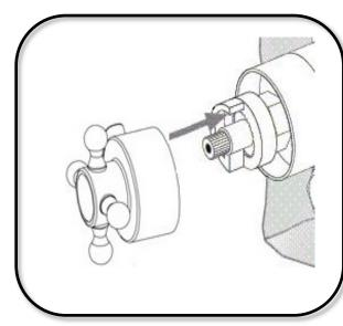
Fit temperature control handle to thermostat, ensuring the stop pin inside the handle, is located against the top of the stop ring.
